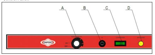
A: Plate resistance on/off / temperature setting
