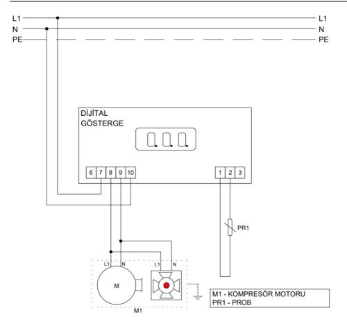
M1-COMPRESSOR ENGINE PR1-PROBE
